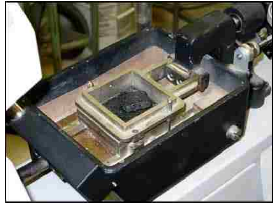
(b) Aggregate pull-off due to shear
