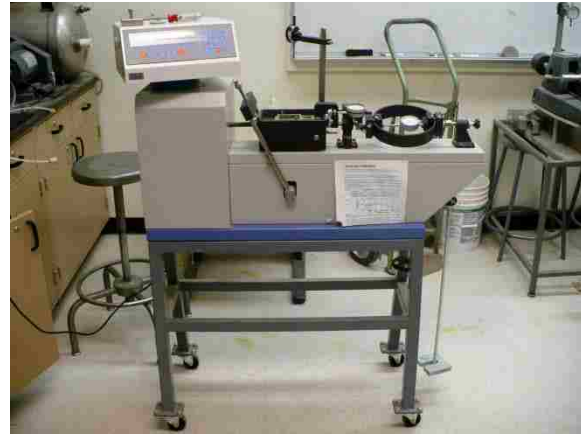
(b) Direct shear test setup
