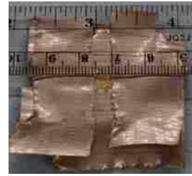
(b) Aggregate covered with duct tape
