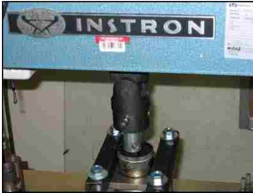
(a) Aggregate pull-off due to tension
