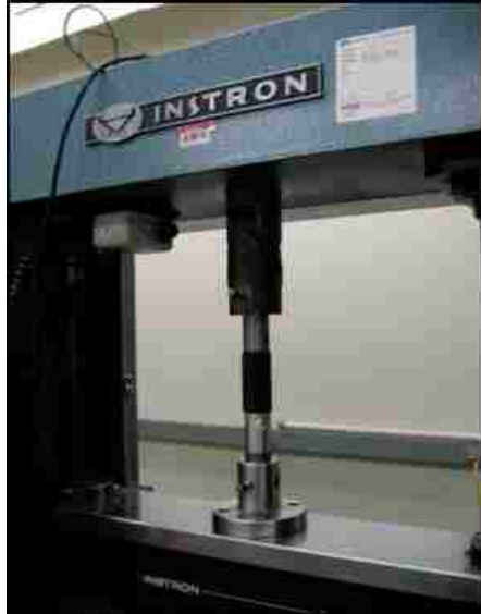
(a) Sample under compression test
